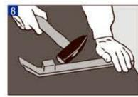
The last row of planks is rounded on the side with the pull bar and on the front side with the tapping block.
